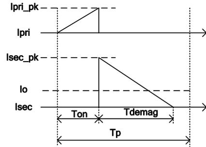
Fig.1 The current waveform in DCM mode
