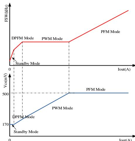
Fig.2 The Switching Frequency, V<sub>CS</sub> VS. LOAD
