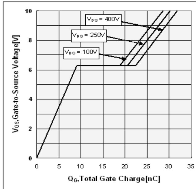
**Fig 6. Typical Gate Charge Vs. Drain-to-Source Voltage**
